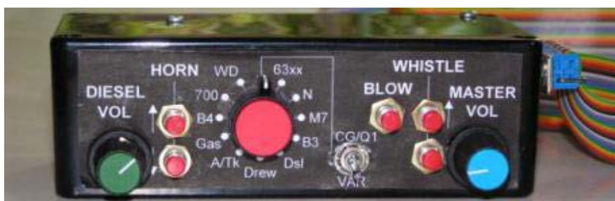
Figure 6. Rotary switch that selects the pre-set resistor values for chuff start-voltage, rate and cut-off.
